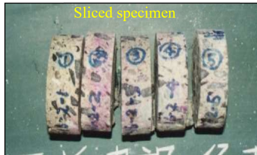
Photo2.6.4 Core sampling status and depth-sliced core samples
