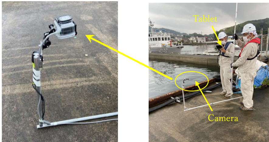
Photo 2.2.4 Example of a hanging camera capable of underwater photography
